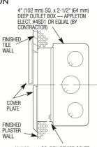
4" (102 mm) SQ. BOX DEVICE COVER (PLASTER RING) 3/4" (19 mm) HIGH — APPLETON ELECT. #8470 OR EQUAL (BY CONTRACTOR)
