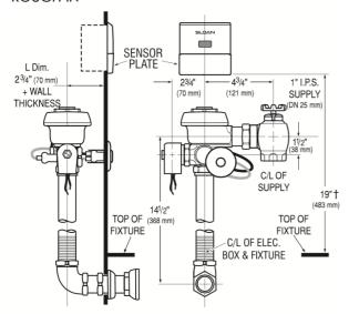
† Position of Sensor Box can be raised or lowered 1" (25 mm) if in conflict with Handicap Grab Bars.
