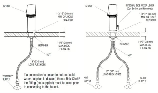
When the BASYS Series faucet is installed on a sink that has three (3) hole punchings, a Base Plate should be used. Base Plates should be specified at time of order.
