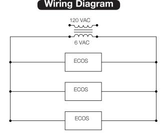
One EL-386 Transformer serves one (1) Optima Closet/Urinal Flushometer. One EL-451 Transformer serves up to six (6) Optima Closet/Urinal Flushometers.
