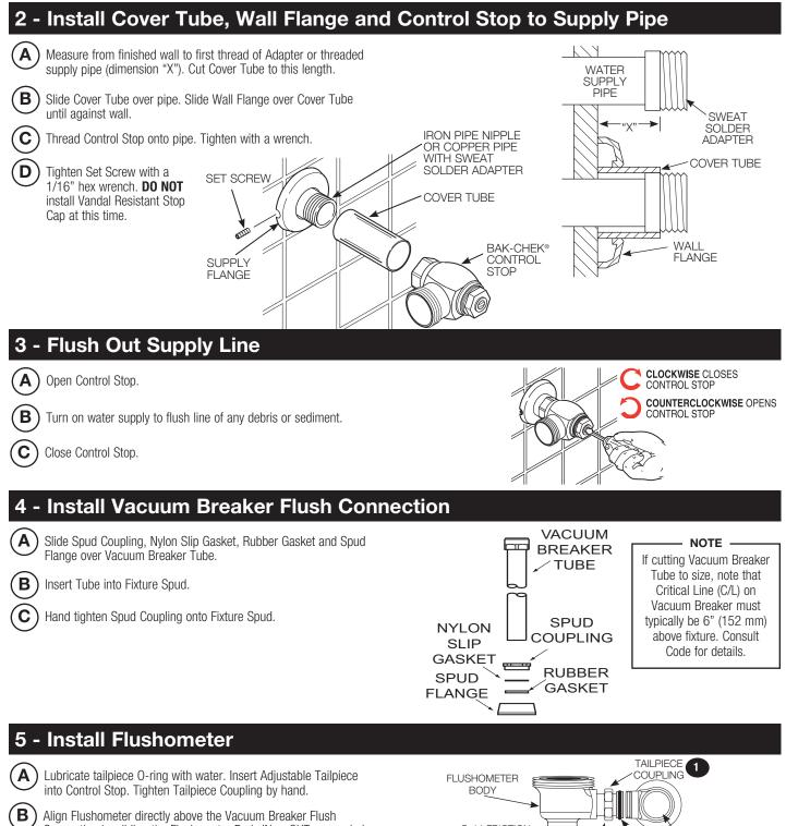
Connection by sliding the Flushometer Body IN or OUT as needed. Tighten Vacuum Breaker Coupling by hand.
