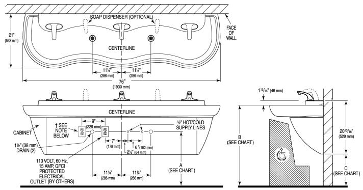
† An additional electrical outlet is required when installing three (3) ETF Faucets.
