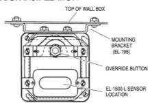
Adjust the Mounting Bracket so that the Sensor sits flush against the Cover
