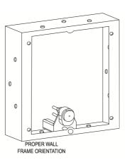
† Position of Sensor Box can be raised or lowered 1" (25 mm) if in conflict with Handicap Grab Bars.
