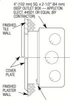
4" (102 mm) SQ. BOX DEVICE COVER (PLASTER RING) 3/4" (19 mm) HIGH — APPLETON ELECT. #8470 OR EQUAL (BY CONTRACTOR)
