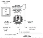
One 50 VAC Transformer serves up to ten (10) OPTIMA Closet/Urina Flushometers. Specify number of transformers required accordingly.
