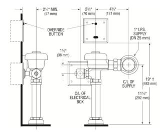
† Position of Sensor Box can be raised or lowered 1" (25 mm) if in conflict with Handicap Grab Bars. 1. A continuous, invisible light beam is emitted from the OPTIMA® Sensor.
