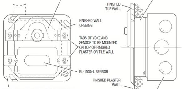
Failure to properly position the electrical boxes to the plumbing rough-in will result in improper installation and impair product performance. All tradesmen (plumbers, electricians, tile setters, etc.) involved with the installation of this product must coordinate their work to assure proper product installation. Installation Template furnished with Flushometer.
