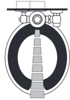
2. As the user enters the beam's effective range (22" to 42") the beam is reflected into the OPTIMA® Scanner Window and transformed into a low voltage electrical circuit. Once activated, the Output Circuit continues in a "hold" mode for as long as the user remains within the effective range of the Sensor.
