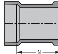
For connection to Cast Iron system. Requires packing and plastic lead.
