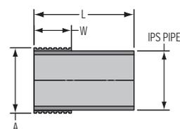
For connection to Duriron® system. Requires Duriron® mechanical joint coupling.
