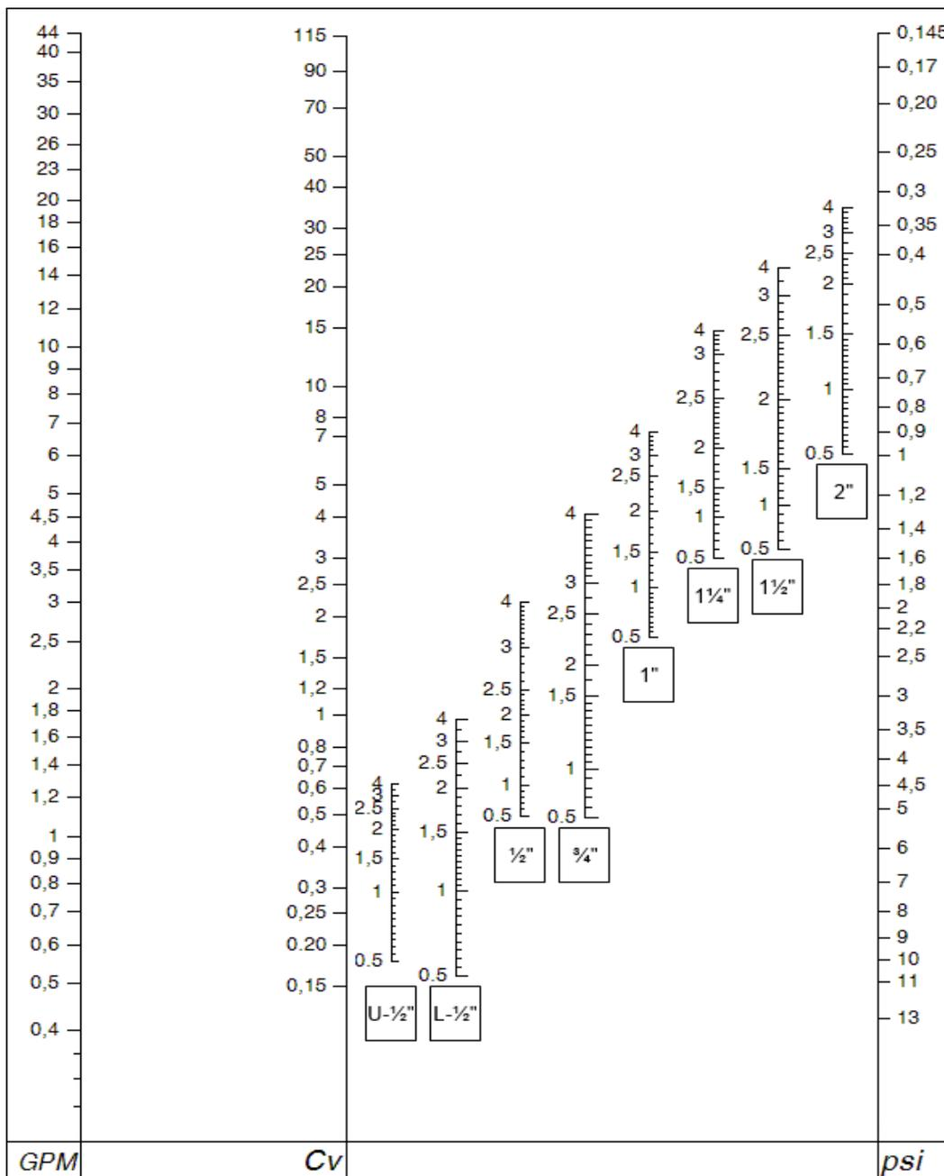
Using the diagram above, it is possible to determine the presetting position of the valve with the given design flowrate and headloss:
