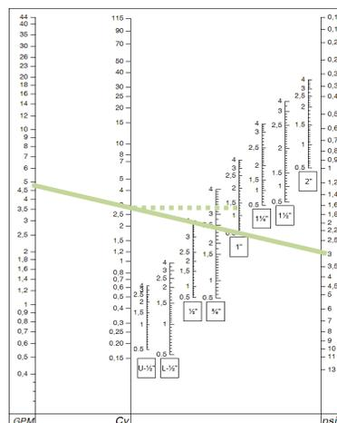
In the example for a design flowrate of 5GPM and design  $\Delta p$  3psi handwheel position of 1.35 is determined for a 1" valve
