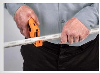
**Step 1**Cut the desired length of pipe.
