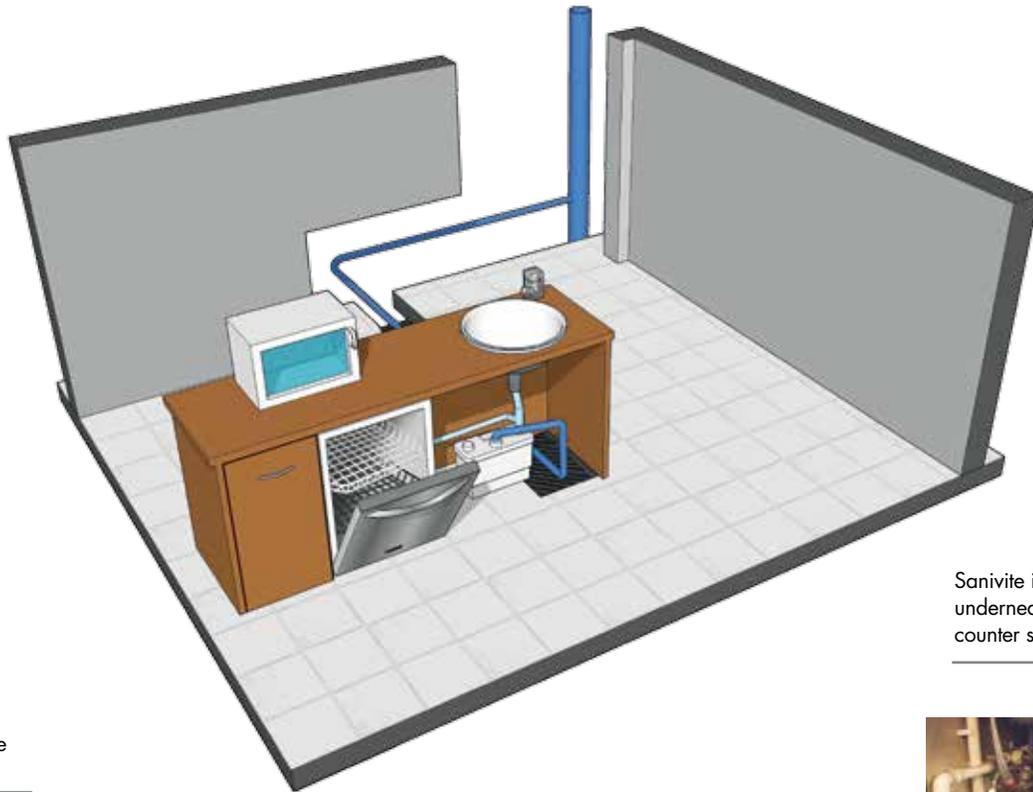
Sanivite installed underneath the counter sink
