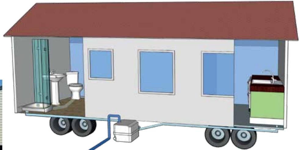
Drain pipe from trailer leading into a Sanicubic 1 grinding system
