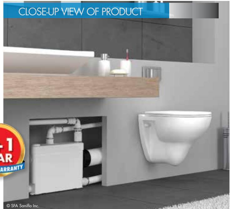
The **Sanipack** is a **1/2 HP pump system** used to install a complete bathroom up to **15 feet below the sewer line, or even up to 150 feet away** from a soil stack. It incorporates a **macerating system** which can handle human waste and toilet paper in residential applications. The blade is made out of a hardened stainless steel material **which eliminates the need for any service or replacement.**
