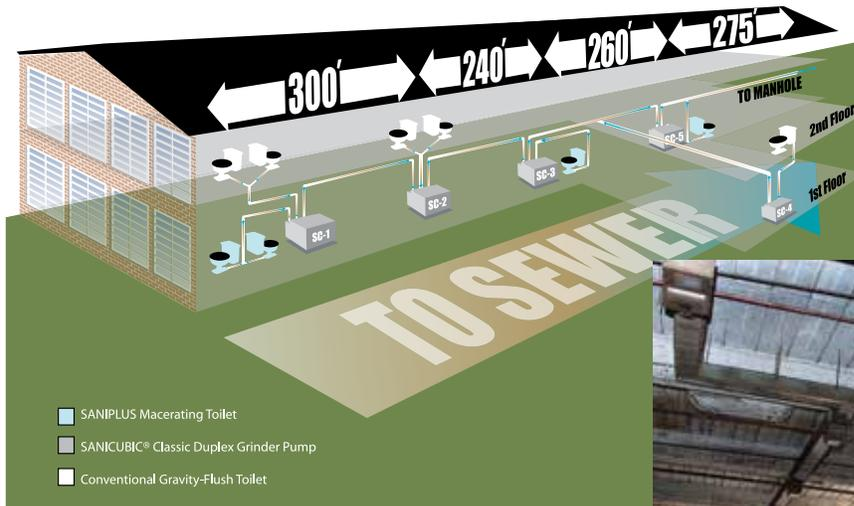
Over 900 feet of horizontal discharge pipe throughout the ceiling of the entire building
