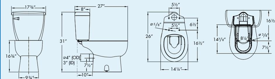
Technical drawings for the round front toilet (Part No. 083) showing dimensions in inches:
