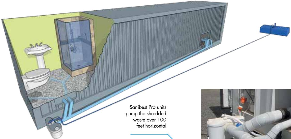
Sanibest Pro units pump the shredded waste over 100 feet horizontal
