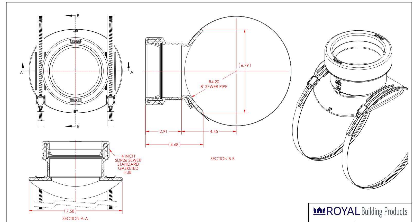
8" SDR26 SEWER REHAB SADDLE TEE & SDR26 SEWER GASKETED HUB SOLVENT WELD SKIRT w/o LOCATING RIB 8" SADDLE x 4" GSK HUB
