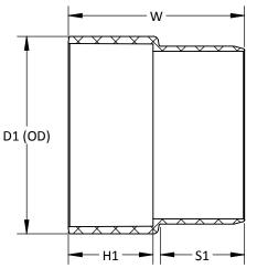
ASTM D3034, CSA B182.2 ASTM D2665, F2135, F1866, CSA B181.2 WHERE APPLICABLE
