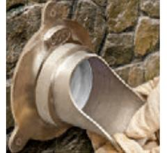
Solvent weld nozzle onto pipe and into escutcheon. *Dura G-O-N requires the mounting notch in the escutcheon and the nozzle be aligned for proper contact.*
