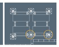
Equipment Clamps are moveable and located on both sides of the cross-bars. Clamps lock down onto the feet of the equipment units as they are tightened.
