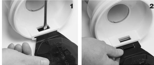
**Remove flapper: 1.** With a flathead screwdriver, push down through the lower collar mount to the bottom clip edge of the flapper insert. Pull old flapper straight back and out.
