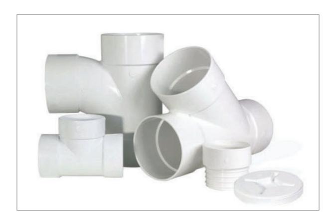
4" through 12" injection molded solvent weld SDR26 sewer fittings shall be manufactured in accordance with ASTM D3034, and CSA B182.2. They shall be injection molded from virgin PVC compound having a cell classification of 12454 or 13343 in accordance with ASTM D1784.
