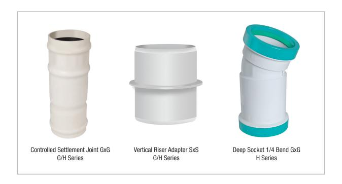
Vertical Risers for Sewers shall contain a Controlled Settlement Joint, a Vertical Riser Adapter, and a Deep Socket fitting. SDR26 pipe and other SDR26 fittings are required for directional and transitional connections. Controlled settlement joints used in a vertical riser system shall provide a minimum of 5½" of axial movement when forces of 500 pounds or greater are applied and shall be fabricated from pipe which is manufactured to ASTM D3034 specifications.
