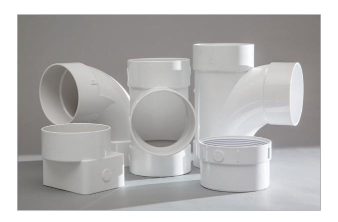
4" through 12" injection molded solvent weld SDR35 sewer fittings shall be manufactured in accordance with ASTM D3034 and CSA B182.2. They shall be injection molded from virgin PVC compound having a cell classification of 12454 or 13343 in accordance with, and certified by the National Sanitation Foundation (NSF), to meet ASTM D1784.
