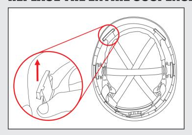
1. Remove the harness by placing your hand on the underside 2. Repeat this process for all 6 clips then take the suspension 3. Place the new suspension inside the hard hat then click of the clip and pushing upwards and towards the back or front of the hard hat until it slides out of place.
