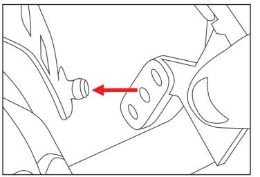
2. To adjust the height, un-pop the arm from the receiver (hold the hard hat and receiver firmly whilst doing so).
