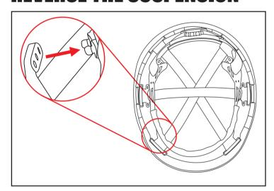
1. Remove the suspension by un-popping the arm from the receiver (hold the hard hat and receiver firmly whilst doing so).
