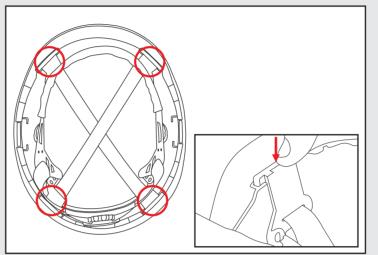
the first clip back down into position. Repeat the process for the 4 main clips.
