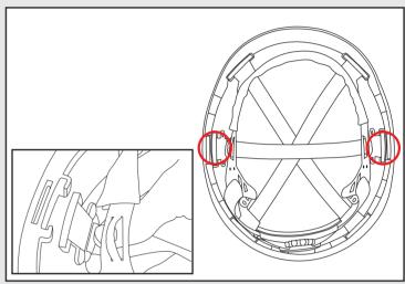
4. Now take the extra strap, thread the first clip between the suspension and the hard hat and click back down. Repeat this for the final clip, making sure that the strap is above the 2 diagonal straps already in place.
