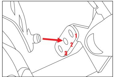
3. Then relocate the arm into 1 of 3 receivers. Repeat this process at all 4 adjustment points.
