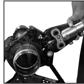
Figure 8: Placement of adapter jaw into pressing chain
