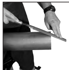
Figure 4: Deburr outside diameter using a half-round file
