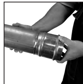
Figure 9: Inspection of final crimp
