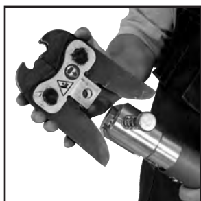
Figure 7: Placement of adapter jaw into the tool
