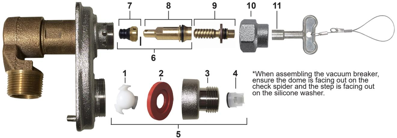
\*When assembling the vacuum breaker, ensure the dome is facing out on the check spider and the step is facing out on the silicone washer.
