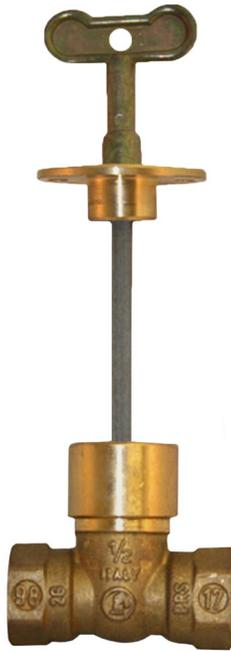
The C-67 AGA Gas Valve is for use on any gas fireplace or appliance. Using the included operating rod, the installer can install the valve from 1" to 14" depth, allowing it to be installed "below-the-joint," eliminating fittings and installation time. The C-67 Gas Valve is also used as a shutoff for any gas burning appliance.
