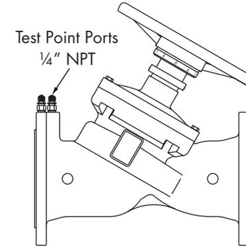
**Fixed Orifice Circuit Balancing Valve**
