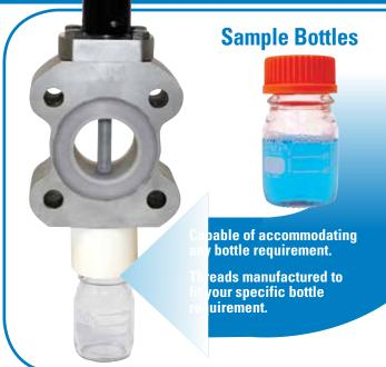
**PRINCIPLES OF OPERATION:** Sampling valves are engineered to effectively collect representative sample of hazardous process media. The dead space free design can be installed in both horizontal and vertical piping, thereby allowing the media to constantly flow through the valve and around the conical spindle. Sample bottles – either open top or sealed with septum, can be directly attached beneath the valve to facilitate the sampling process.
