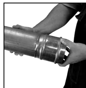
Figure 9: Inspection of final crimp
