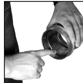
Figure 5: Check for EPDM seal
