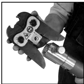
Figure 7: Placement of adapter jaw into the tool
