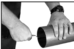
Figure 3: Deburr inside diameter deburring tool
