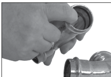
Figure 2 — Check for EPDM Seal
