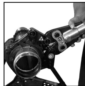
Figure 8: Placement of adapter jaw into pressing chain
