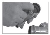
Figure 2 — Check for EPDM Seal
