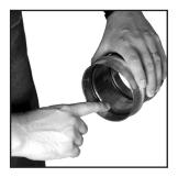
Figure 5: Check for EPDM seal
