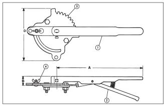
The position-lock can be used to set the valve in any position or as a memory stop so the valve may be reopened to the previous position. The valve may be padlocked in full open or full closed position.
