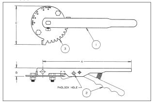
The lever-lock handle and throttling plate provide throttling notches every 10<sup>0</sup> for excellent manual control in balancing up to 90<sup>0</sup> or shut off service. The valve may be padlocked in any one of the positions including opened or closed by virtue of a locking hole located in the handle and lever.
