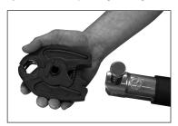
Figure 5 — Inserting the NIBCO Press System jaw
