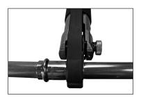
Figure 8 — Jaw set should be square to tubing
