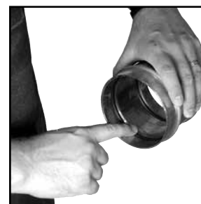
Figure 5: Check for EPDM seal
