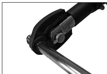
Figure 7 — Open the jaw set and place around the fitting
