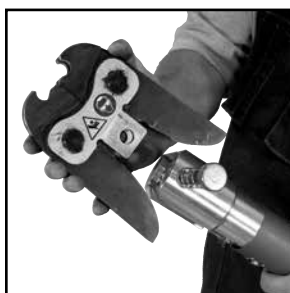
Figure 7: Placement of adapter jaw into the tool
