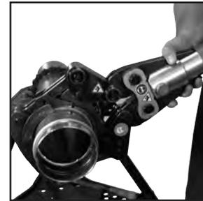
Figure 8: Placement of adapter jaw into pressing chain
