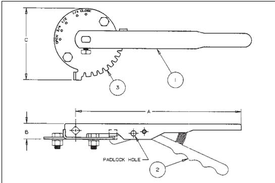
The lever-lock handle and throttling plate provide throttling notches every 10° for excellent manual control in balancing up to 90° or shut off service. The valve may be padlocked in any one of the positions including opened or closed by virtue of a locking hole located in the handle and lever.
