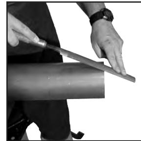
Figure 4: Deburr outside diameter using a half-round file
