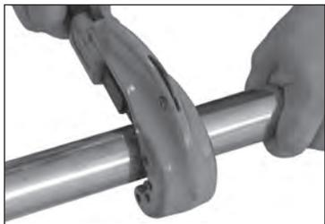
Figure 1 — Cut tube to desired length
