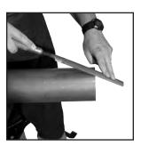
Figure 4: Deburr outside diameter using a half-round file
