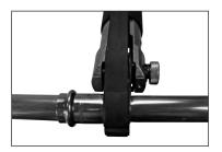
Figure 8 — Jaw set should be square to tubing
