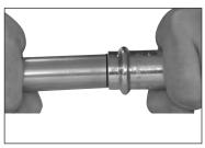
Figure 6 — Inserting the tube to proper depth
