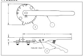
The lever-lock handle and throttling plate provide throttling notches every 100 for excellent manual control in balancing up to 900 or shut off service. The valve may be padlocked in any one of the positions including opened or closed by virtue of a locking hole located in the handle and lever.
