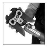
Figure 7: Placement of adapter jaw into the tool
