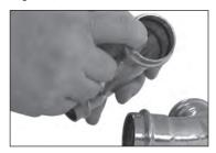
Figure 2 — Check for EPDM Seal
