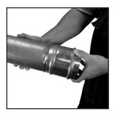
Figure 9: Inspection of final crimp
