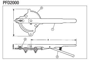
The position-lock can be used to set the valve in any position or as a memory stop so the valve may be reopened to the previous position. The valve may be padlocked in full open or full closed position.
