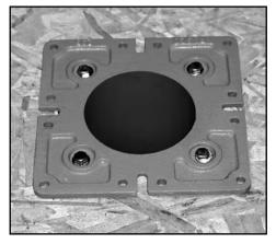
**PASCO**'s NEW Quick Set Square Closet Flange will solve the problem of properly supporting a closet flange mounted in a square hole. Keep in mind that the pipe doesn't support the flange, the sub-floor does. Simply push the QUICK SET CLOSET FLANGE flush on the DWV pipe and alternately tighten the flour stainless steel screws. Secure to subfloor with brass wood screws.
