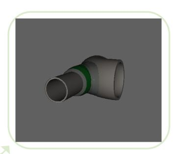
Equation for overall length  $L = E + \sqrt{B^2 - A^2} + Root gap$
