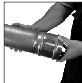
Figure 9: Inspection of final crimp
