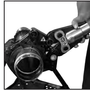
Figure 8: Placement of adapter jaw into pressing chain
