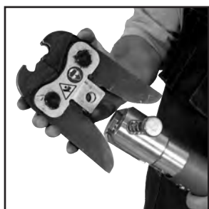
Figure 7: Placement of adapter jaw into the tool
