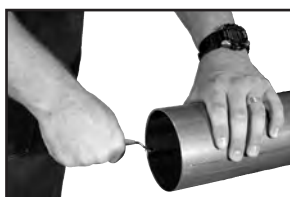
Figure 3: Deburr inside diameter deburring tool
