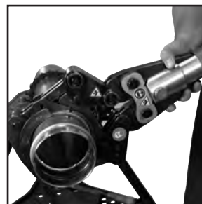
Figure 8: Placement of adapter jaw into pressing chain
