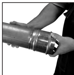
Figure 9: Inspection of final crimp
