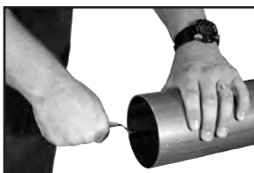
Figure 3: Deburr inside diameter deburring tool
