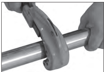
Figure 1 — Cut tube to desired length
