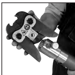
Figure 7: Placement of adapter jaw into the tool
