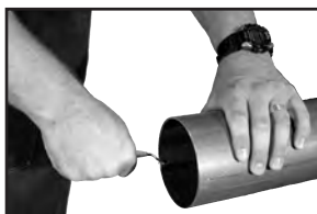
Figure 3: Deburr inside diameter deburring tool
