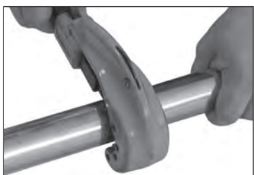
Figure 1 — Cut tube to desired length
