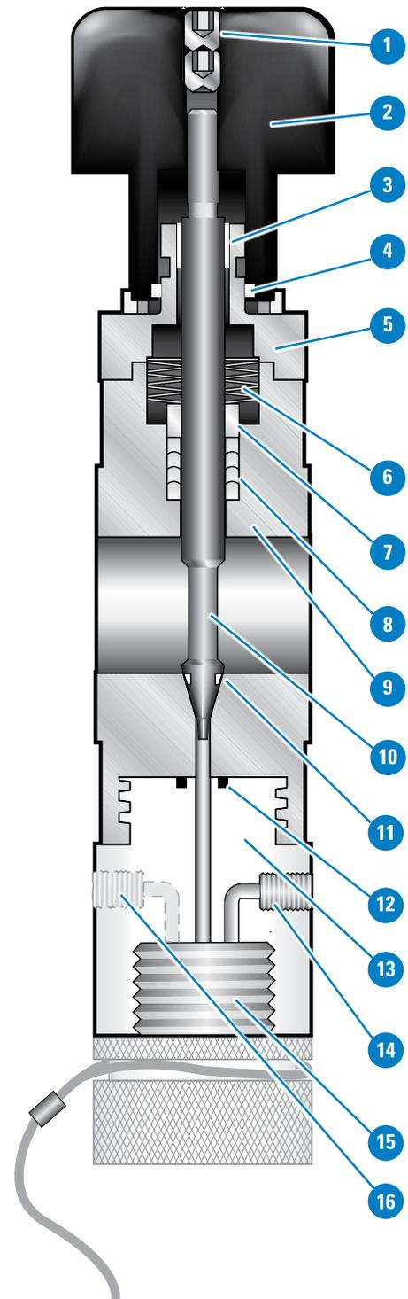
**PRINCIPLES OF OPERATION:** Sampling valves are engineered to effectively collect representative sample of hazardous process media. The dead space free design can be installed in both horizontal and vertical piping, thereby allowing the media to constantly flow through the valve and around the conical spindle. Sample bottles – either open top or sealed with septum, can be directly attached beneath the valve to facilitate the sampling process.
