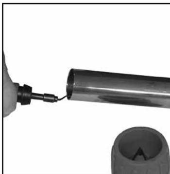
2. Deburr the tube inside diameter using a rounded file or a deburring tool.
