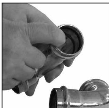
4. Check the fitting to make sure that the seal is in place, clean and free of contaminants. Only original NIBCO EPDM seals are to be used when making press connections with NIBCO Press System fittings and valves. If it is necessary to lubricate the seals, use water only. Do not use any petroleum-based lubricants.
