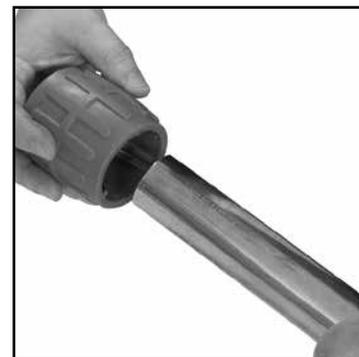
3. Deburr the tube outside diameter using a rounded file or a deburring tool. Clean the tube end of all dirt, oil and grease as well as copper dust and chips from sawing.
