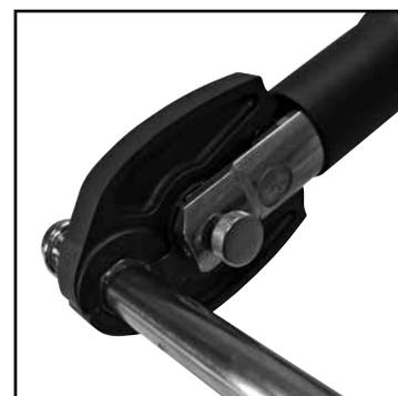
6. Ensure that the proper pressing jaws are installed in the pressing tool and squeeze jaw arms to open jaw set. Place open jaws around the fitting end and ensure that the contour of the jaw is properly aligned with the contour of the fitting. Make sure the tube is inserted to the proper depth in fitting (reference mark from #5) and with the tool at a right angle to the tube, start pressing procedure.
