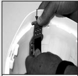
**STEP3:** Place the other end of the strap in the opposite connection slot at the rear on the right hand side with the helmet facing forward. Push the clip downwards until you hear a click, making sure the tail is facing towards the front of the helmet.
