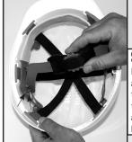
**STEP 9:** Pick up the wheel ratchet labelled 5 in step 1. Locate the two holes at the rear of the head piece and push the two pins on the wheel ratchet through the holes. Repeat on the other side to attach the wheel ratchet and complete the barreers.
