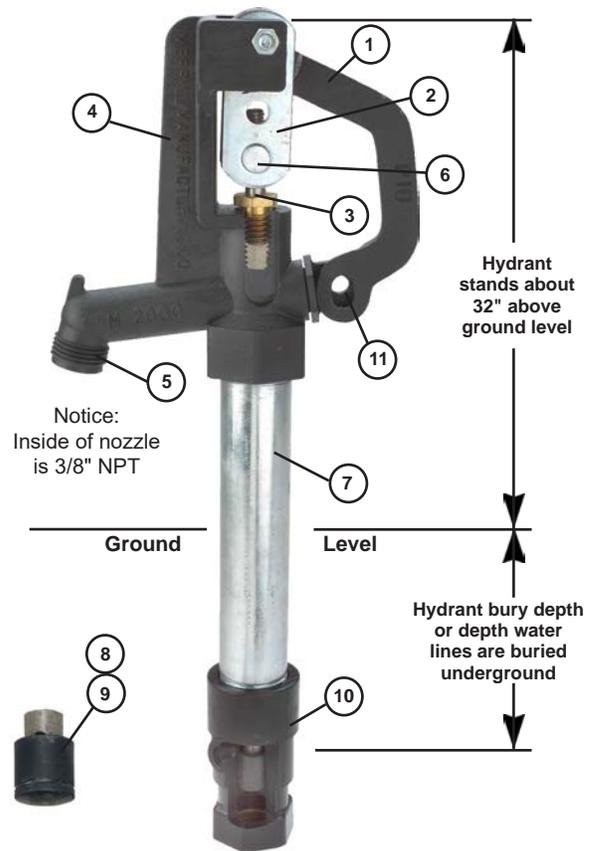
Merrill's MP7504 or 4' bury hydrant is 6' - 8' long, 4' is buried and 32" above ground.
