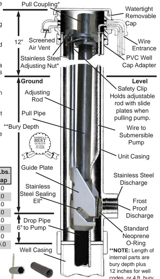
**\*\*NOTE:** Length of internal parts are bury depth plus 12 inches for well codes, or 4 ft. bury is approximately 5.5 ft. long. Custom wrenches for stainless steel adjusting nut available from Merrill.
