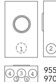
200 amp | 4 Terminal | Ringless | Jaw Clamping Lever Bypass | Single Position | 1Ø3W or 3Ø3W
