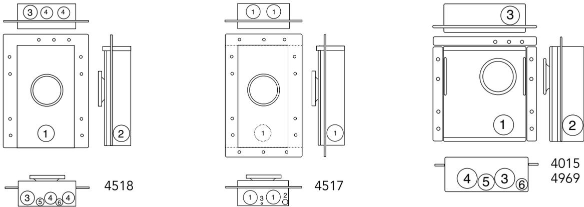
200 amp | 4 Terminal | Flush Mount | Ring Type | Single Position
