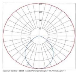
Maximum Candela = 289.05 Located At Horizontal Angle = 180, Vertical Angle = 1 # 1 - Vertical Plane Through Horizontal Angles (180 - 0) (Through Max. Cd.)
