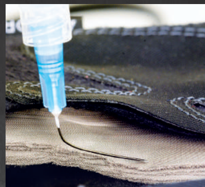
25 gauge needle failure
