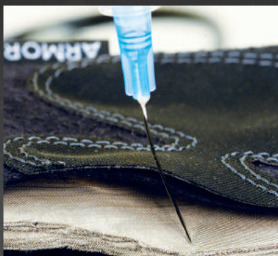
25 gauge needle buckling
