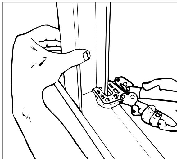
Metal Stud Crimper. Secures metal stud and runner without fasteners.
