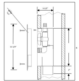
Note: For boxes containing only 1-valve, left hand side valve & supply hole are omitted.
