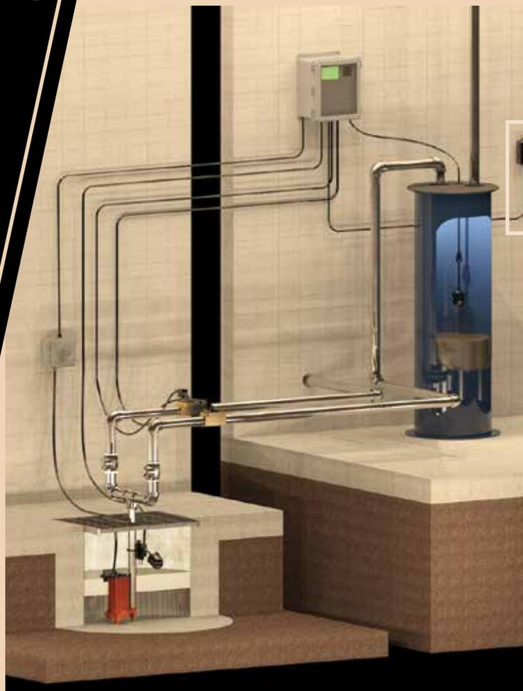
In the event of an oil leak, the spilled oil will collect in the sump and float on the surface of the water. Once the layer is thick enough to trip the high oil float, the pump will eliminate the oil and water in the sump; the water will be pumped to the drain and then the oil will be routed to the waste oil storage tank preventing unwanted contamination.
