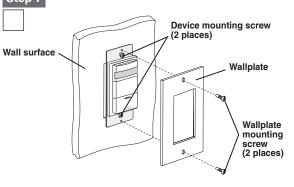
Secure device by firmly tightening mounting screws.
