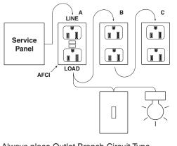
Always place Outlet Branch Circuit Type AFCI in position A. All outlets of the protected branch, including lighting and receptacle outlets must be connected to the load side of the AFCI.
