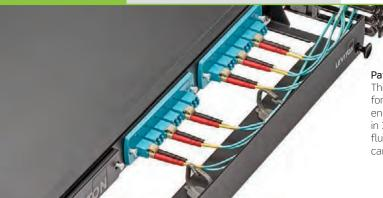
**Patch Cord Management Trays** help route and organize cables. The trays feature identification labels and front saddles that pivot for easier routing. Because they mount directly to the front of the enclosures, they do not require additional rack space. Available in 1RU and 2RU sizes, the trays can be used with any Leviton 1RU flush-mount MTP enclosure or e2XHD flat panel, and 2RU trays can be used with 3RU 500i SDX enclosures. **See page B22.**
