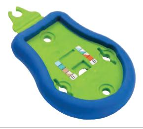
Use the Leviton Palm Termination Tool (page A44) to quickly and easily punchdown jacks at the job site. The Palm Termination Tool was designed with installer input and offers an ergonomic comfort grip, increased jack stability, and integrated holes that allow rack mounting for QuickPort panel terminations. The Palm Termination Tool is compatible with eXtreme™ Cat 6A/6/5e, GigaMax™ Cat 5e, and QuickPort AV jacks.
