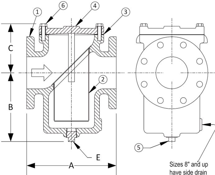
Sizes 8" and up have side drain blow-off hole.
